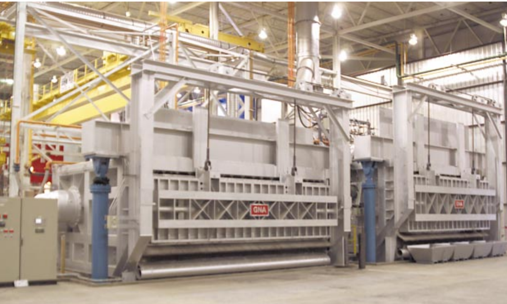
50 ton tiltable holding furnace
